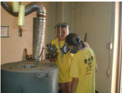
Figure 1. Chelsie is looking at molten metal in a container where we soon put our Styrofoam nosecones. The nosecones were packed into sand, and then the metal was poured on top of it. The metal melted the Styrofoam away, causing it to mold into the nosecone shape. Melanie is reading the temperature of the metal. It turned out to be about 1525 degrees.
